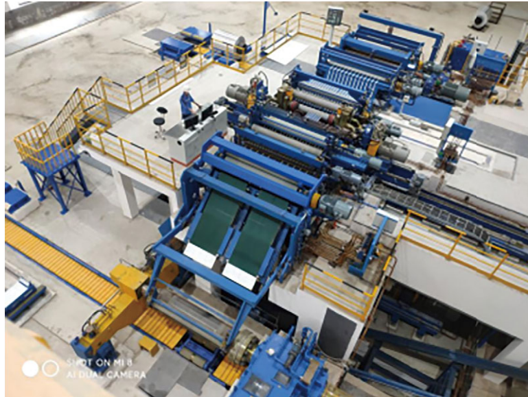
2,300mm aluminum strip high-speed trimming line
